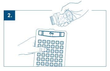
Quantification: For quantitative testing pour the 100 ml sample into the COLIKAT Enumeration Tray. COLIKAT RAPID® turned yellow coliforms are present. If it shows fluorescence under UV-light Escherichia coli is present.
