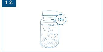
For presence/absence testing incubate the closed vessel for 18-22 hours at 36°C ± 2°C and read-off the result. The vessels should have room temperature before incubation. If turned yellow coliforms are present. If it shows fluorescence unter UV-light Escherichia coli is present.
