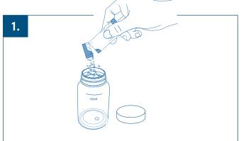
Presence/ Absence: Add 1 bag of COLIKAT RAPID® to 100 ml of water sample. Close the sample vessle and shake until the reagent dissolves.
